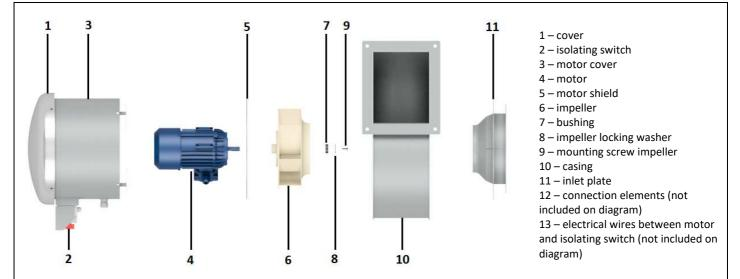
Casing (10), motor shield (5), motor cover (3) and inlet plate (11) are made from painted carbon steel. Cover (1) is made from aluminum sheet. Impeller (6) is made from aluminum or steell depending on the model. Bushings and connection elements (7, 8, 9) are made from steel, galvanized steel, stainless steel. For sealing - sealing paste and or sealing tapes (e.g. EPDM) has been used. Full list of components and materials used in fan can be provided on reasonable request.
